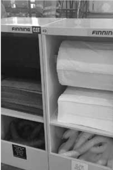
Spill kits are required at all facilities and are inspected and replenished regularly.
