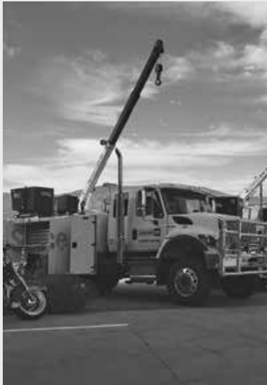
Trucks with power packs consume 30-35% less diesel than regular trucks by reducing idling to run ancillary equipment.
