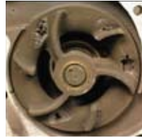
Results using a competitive heavy duty coolant that claimed to meet industry standards. The test score for this coolant was less than 4.
