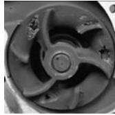
Results using a competitive heavy duty coolant that claimed to meet industry standards. The test score for this coolant was less than 4.
