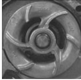
Cat® NGEC™ protected this water pump and earned a nine out of ten on the test.
