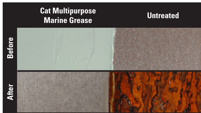
Cat® Multipurpose Marine Grease withstood thousands of hours of salt fog while protecting the metal underneath.
