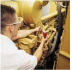
Coolant compartments with sampling valves can be sampled using the same steps as the oil sampling valve method described earlier.
