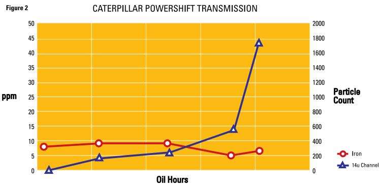
Particle Count has been used for many years by the fluid power industry to monitor debris levels in close-tolerance hydraulic systems. The ability to warn of severe wear across a wide range of materials and micron sizes makes it a useful tool in trending wear debris levels in most equipment compartments, especially hydraulics.
