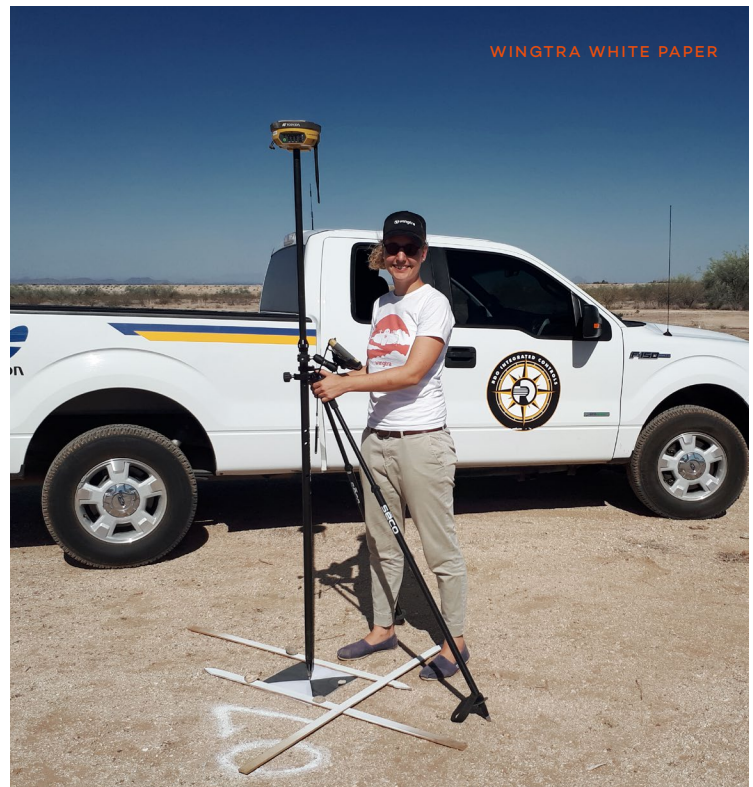
A Topcon HiPer V GNSS antenna was used in the Arizona desert, enabling a centimeter accuracy comparison when testing the WingtraOne.
